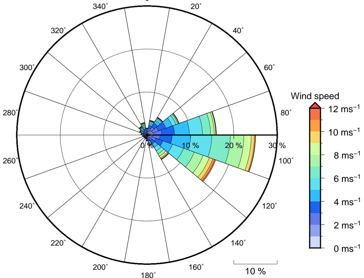
**Figure 11** Annual wind rose for Fugro Directional Wave Buoy. Note that directions are where the wind is coming from.
