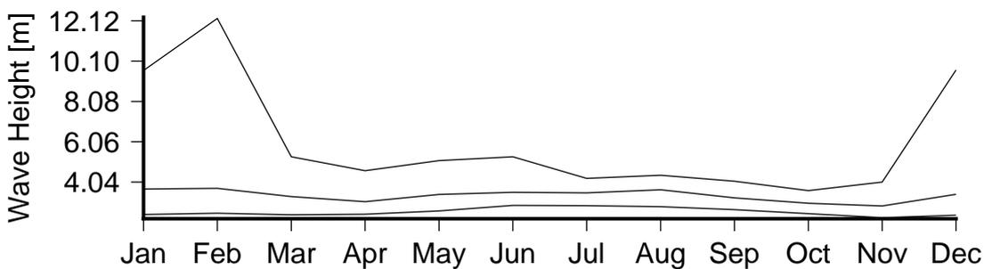
**Figure 7** Monthly variation in large waves (90th percentile)(lower curve), severe waves (99th percentile) (middle curve) and the largest wave(upper curve) in Fugro Directional Wave Buoy.
