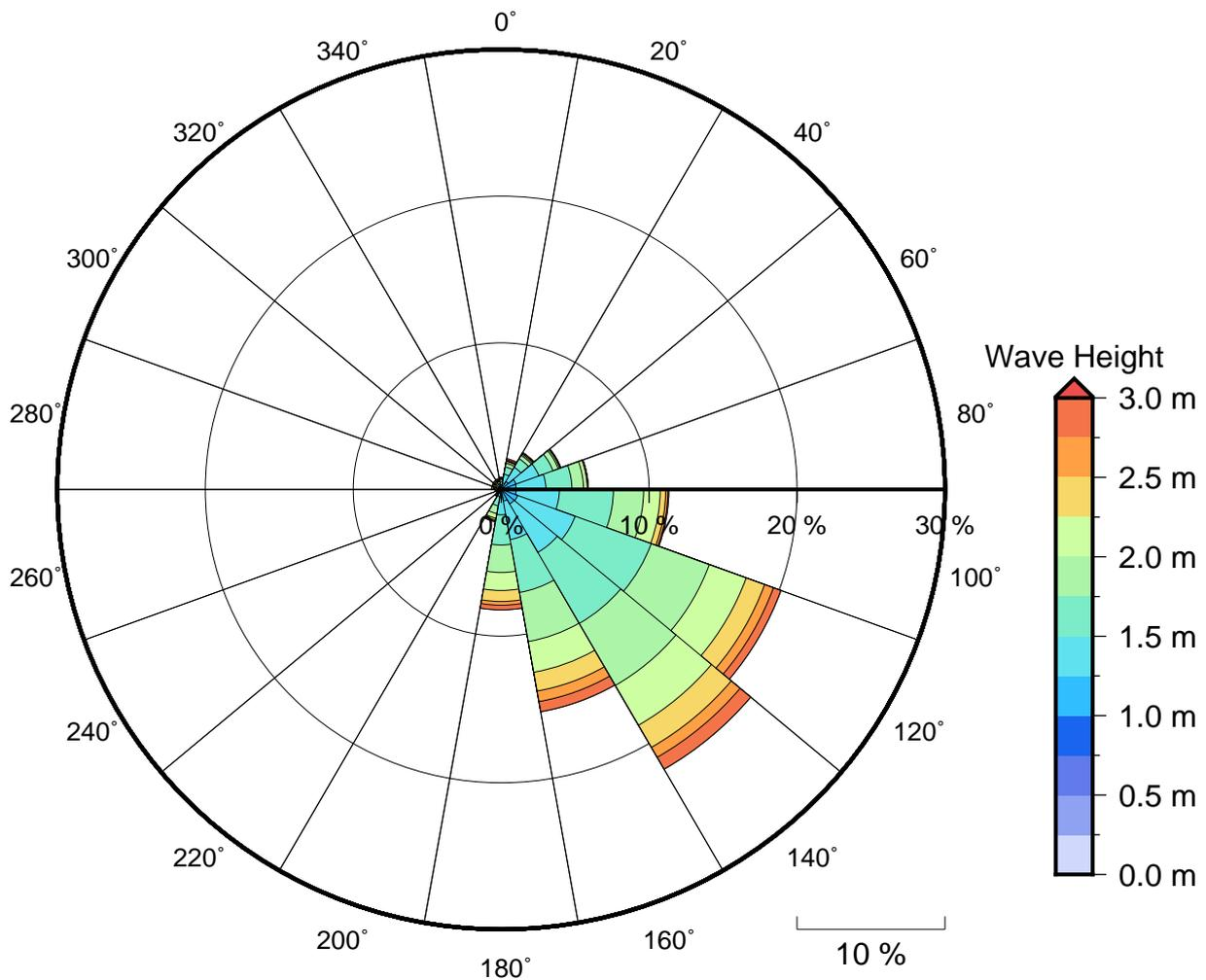
**Figure 2** Annual wave rose for Fugro Directional Wave Buoy. Note that direction are where the wave are coming from.
