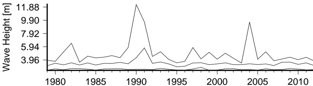
**Figure 8** Annual variation in large waves (90th percentile)(lower curve), severe waves (99th percentile) (middle curve) and the largest wave(upper curve) in Fugro Directional Wave Buoy.
