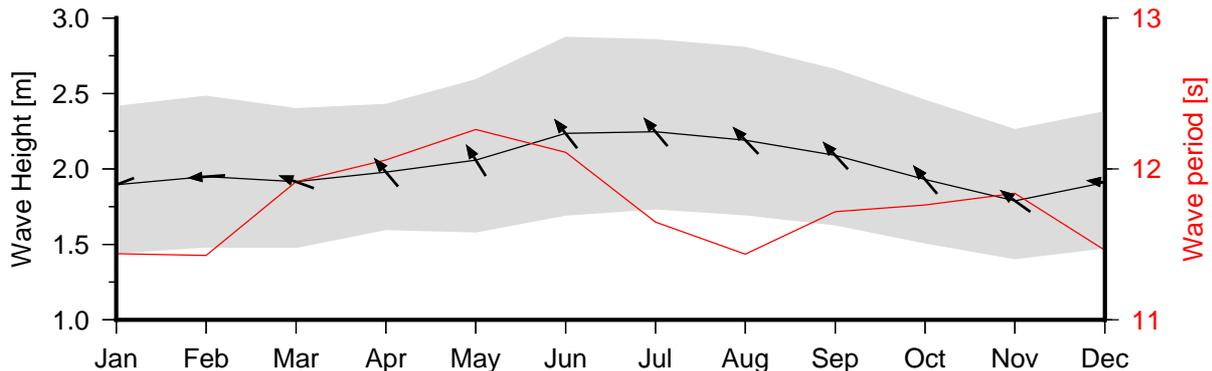
**Figure 4** Monthly wave height (Black line), wave period (Red line) and wave direction (arrows). The grey area represents the range of wave height between calm periods (10% of lowest wave height) and large wave events (10% of highest wave height)
