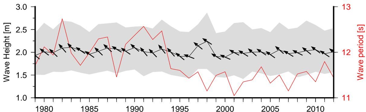
**Figure 5** Annual wave height (Black line), wave period (Red line) and wave direction (arrows). The grey area represents the range of wave height between calm periods (10% of lowest wave height) and large wave events (10% of highest wave height)
