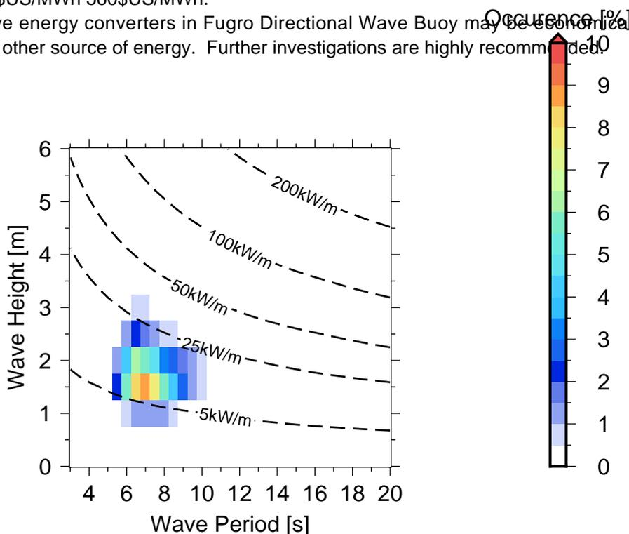
Figure 10 Occurrences of sea states in Fugro Directional Wave Buoy .
