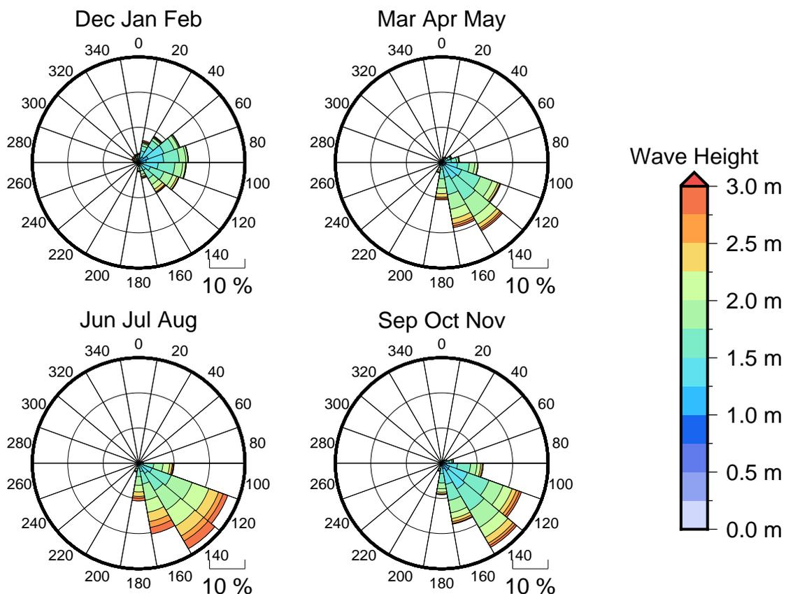
Figure 3 Seasonal wave roses for Fugro Directional Wave Buoy
