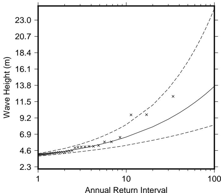
**Figure 9** Extreme wave distribution for Fugro Directional Wave Buoy. The crosses represents the wave events that occurred since 1979. The plain line is the statistical distribution that best fit the past wave events. The dotted line show the upper and lower high confidence of the fit, there is a 95% chance that the fitted distribution lie between the two dashed lines.
