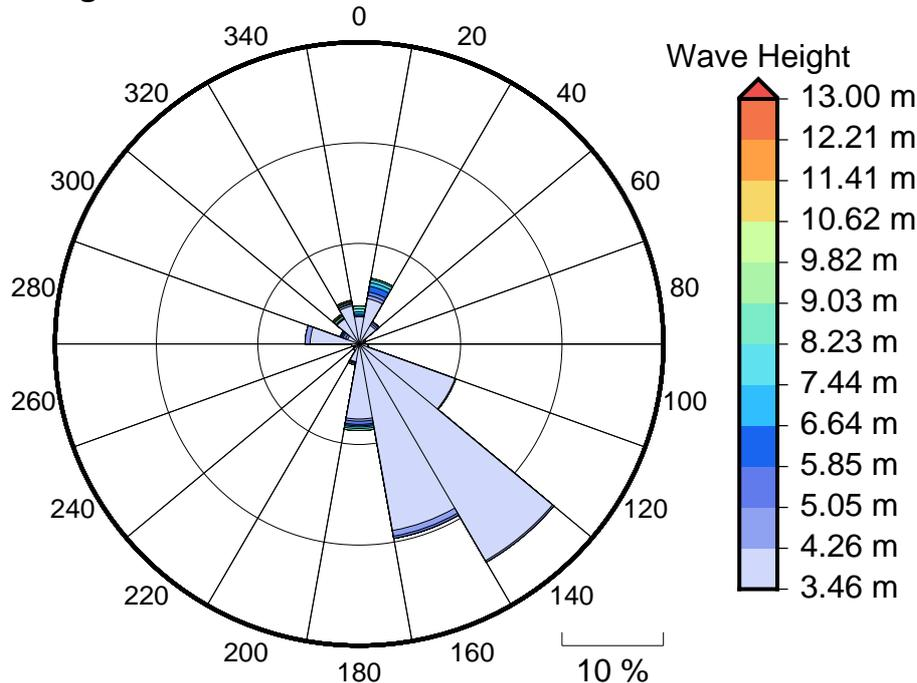
**Figure 6** Large, severe and extreme wave roses for Fugro Directional Wave Buoy
